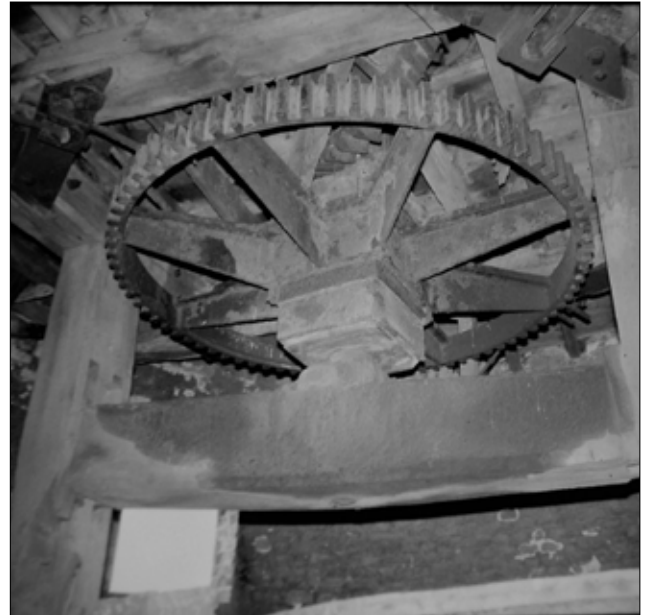
The Great Spur Wheel and associated fittings in 1989. The top of the cover to a pair of mill stones is just visible at the bottom of the picture
